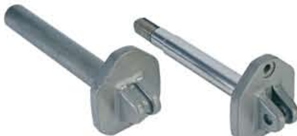
Motion axle Forged blank and finished part
